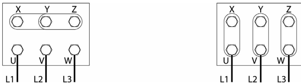
Figure 9. Wye configuration for 400 V voltage (pre-set) Figure 10. Delta configuration for 230 V voltage
